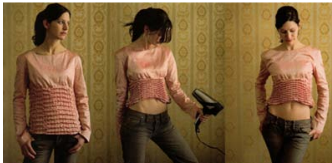
Dutch Designer Mariëlle Leenders developed this shirt using SMA threads woven into the textile.
