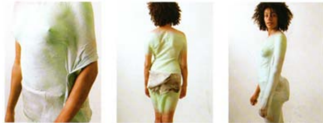
Developed by american designer Manuel Torres, FabriCan consists of spray a material that turns into a nonwoven fiber on the body.
