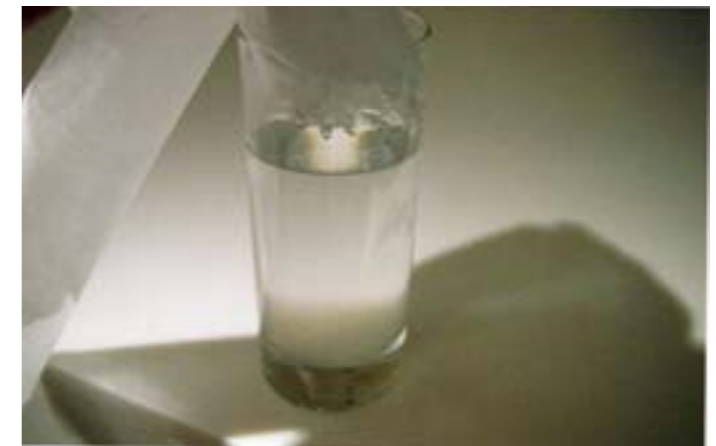
Vilene is a range of interlinings offered by the german manufacture Freudenberg Vliesstoffe FG. It goes from a wide range of light to heavy, as well as high volume nonwovens. The nonwoven interlining dissolves in lukewarm water (25° to 40°C). It is a non-irritating to the skin and offers the option of individually designed garments.
